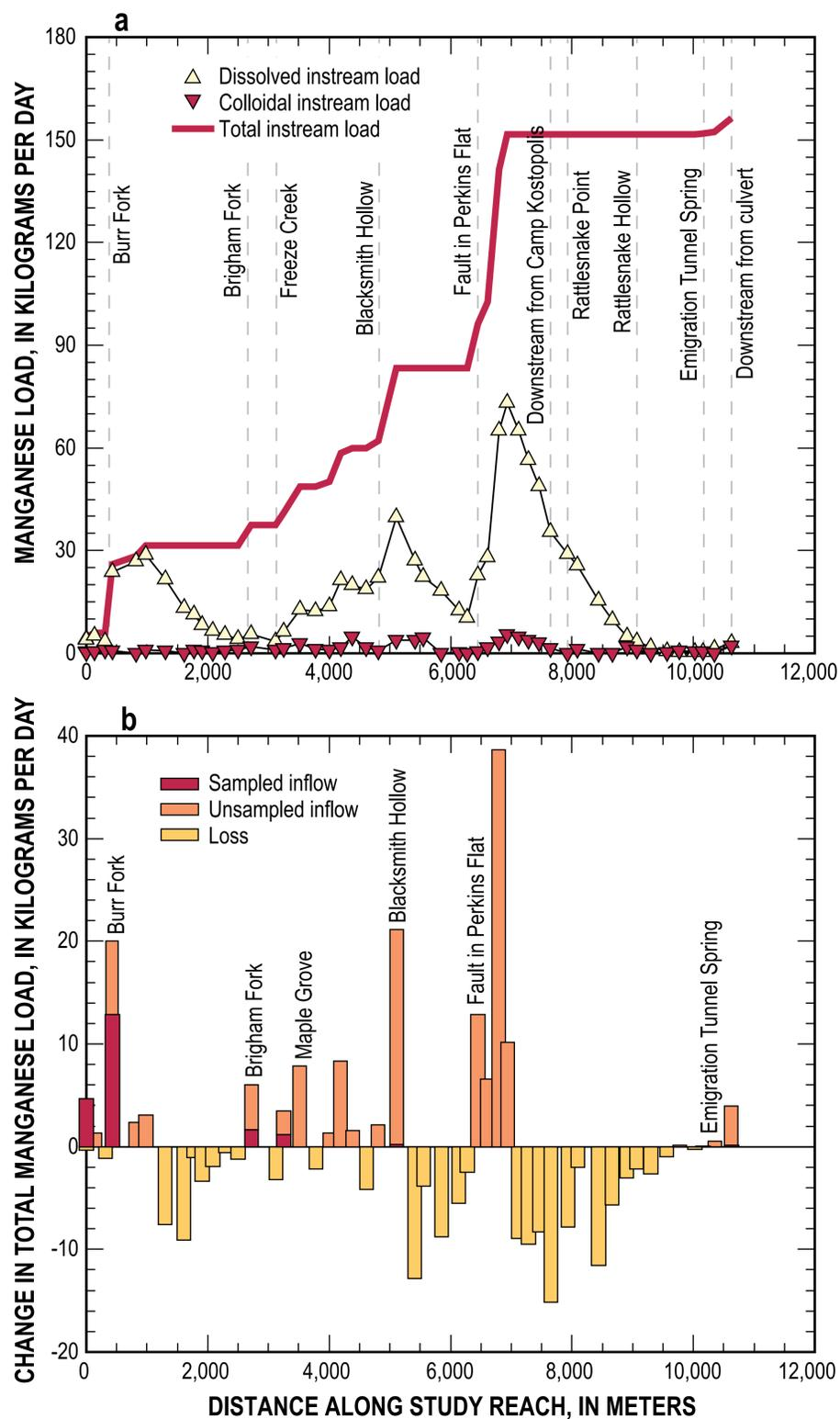
**Figure 12.** Variation of (a) dissolved and colloidal manganese load and (b) change in manganese load for individual stream segments with distance along the study reach, Emigration Creek, Utah, October 12, 2005.
