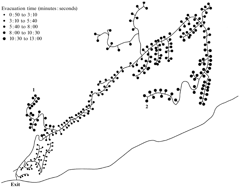
Figure 6. Mean household evacuation travel times for an urgent scenario with high household-vehicle use (mean number of vehicles per household = 2.5, mean departure time per vehicle = 10 minutes).
